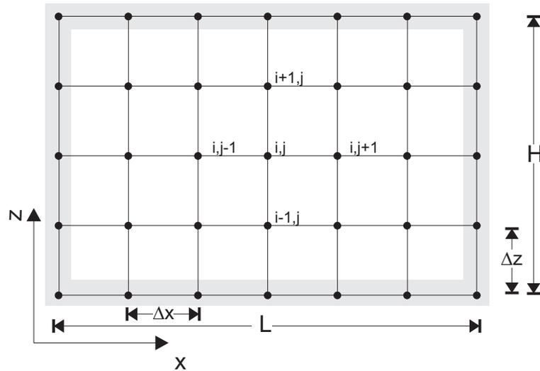
**Figure 1:** Finite difference discretization of the 2D heat problem.
